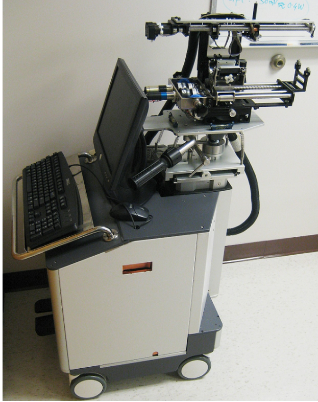
Fig. 1. Single channel image-guided robotic brachytherapy system.
