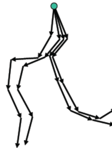
In every step, draw a step direction from the pdf of the underlying fiber orientation.
