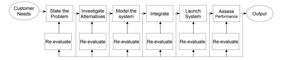
The Systems Engineering Process from A. T. Bahill and B. Gissing, Reevaluating systems engineering concepts using systems thinking, *IEEE Transaction on Systems, Man and Cybernetics, Part C: Applications and Reviews,* **28** (4), 516-527, 1998.
